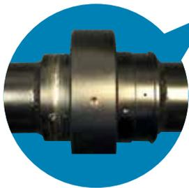
It is important to ensure that the o-ring supplied with the manifold is inserted into the end cap before it is tightened up. The 90-115mm 'C' Spanner (Part No. 35017403, not supplied) is used to assemble the manifold sections and also tighten the end cap.
