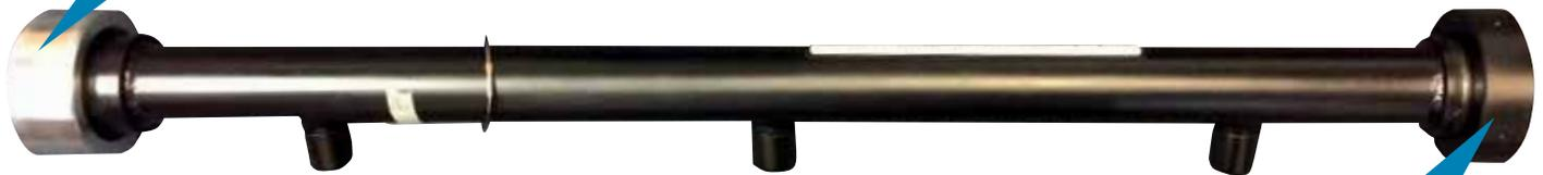
For Manifolds with more than 5 ports, two manifold sections are required to be connected together. For example a 6 port 80L manifold is produced by connecting two 3 port 80L manifolds (Part No. 35116506) together. The end cap must be removed from one of the manifold sections and an o-ring inserted into the female union first:
